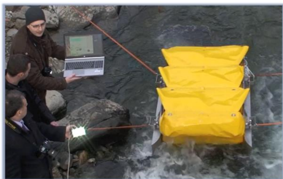
Fig. 10.24 Functional tests on water (Bogorin-Predescu, Țițu, & Țițu, Data acquisition system for a hydroelectric turbine with deformable blades, 2024)
