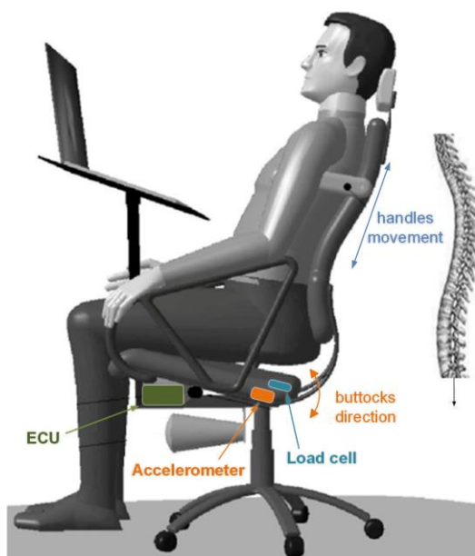
Fig. 9.1 Sketch of the prototype for BI "Chair for working at the PC, with active principle of relaxing the spine" (Romania Patent no. 129280-B1. 2021)
